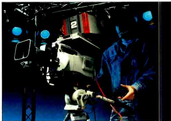
The LDK 10P offers Dynamic Pixel Management (DPM), which provides quick switching between aspect ratios. An automatic dual skin contour system provides precise control over flesh tones and skin quality.
