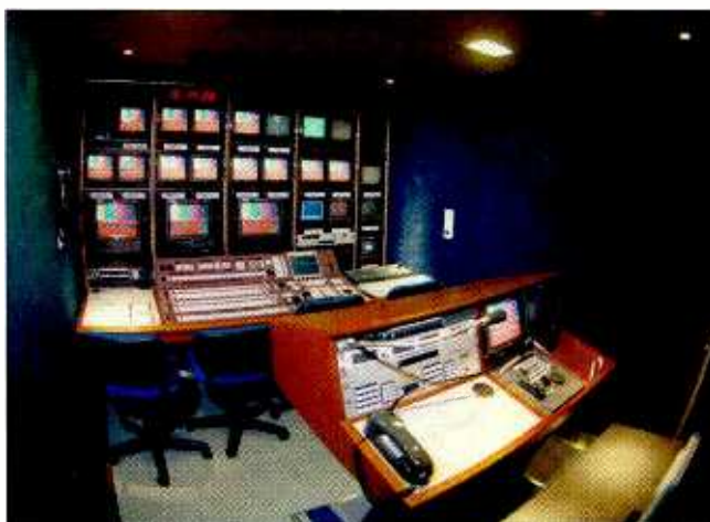
Front section of the truck includes video mix and CG positions (background), plus TD's and slow-motion operator's positions (smaller console in foreground).
