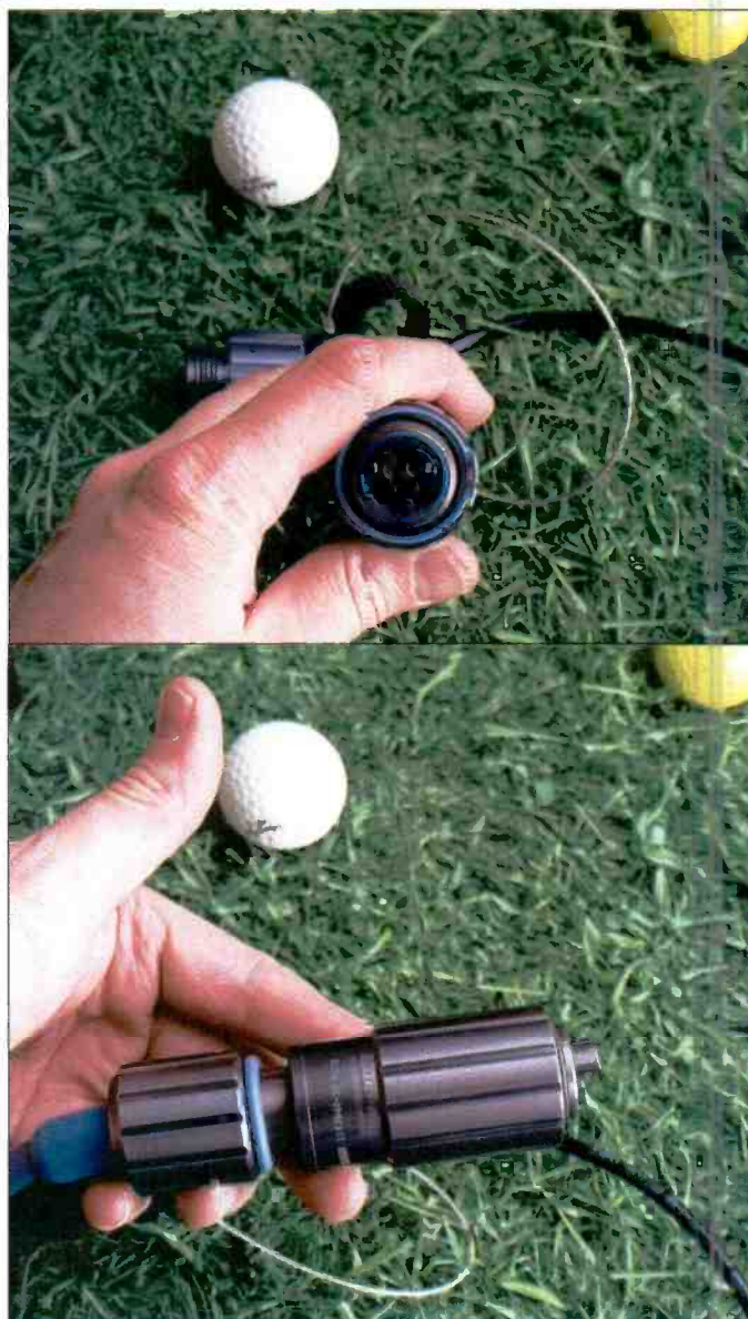
The military multipin hermaphroditic connector handles up to four fibers in a screw-on connector with opposite genders on either end of the cable (like XLR connectors).
