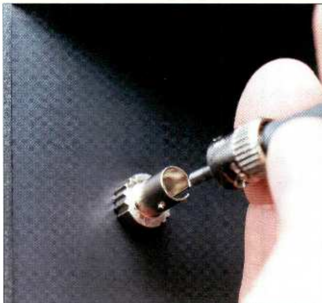
Like BNCs or F connectors on coax, the single-fiber ST connector uses male plugs on all cable ends and female jacks on chassis mounts.
