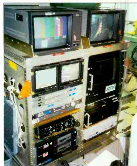
The left bay contains all the video equipment and the right side contains the ACTS antenna tracking computer and audio equipment.
