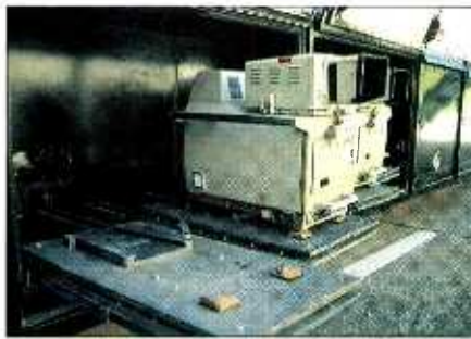
Camera sleds in the belly of the trailer, first sled is partially extended and has camera removed, more sled-mounted cameras are in the background.
