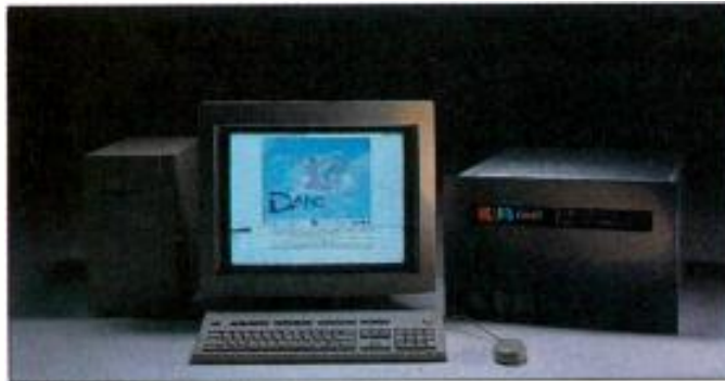
DANCE from KUB Systems includes a Macintosh Quadra with 20-inch display and a dedicated digital video processing box.
