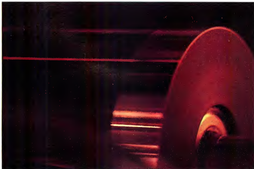
Magnetic coating is scanned for microscopic defects by laser, which counts and pinpoints areas requiring corrective action. (Courtesy of Ampex.)
