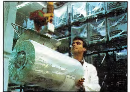
A roll of polyester base film being loaded into machines that will prepare it for coating. (Courtesy of Agfa.)
