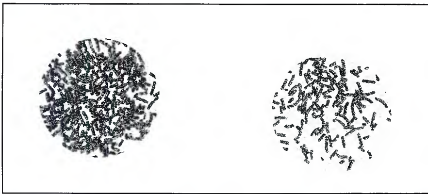
Figure 1. Photomicrographs showing particle densities of metal particle tape (left) and standard ferric oxide tape (right). (Courtesy of DIC Digital Supply Corporation.)
