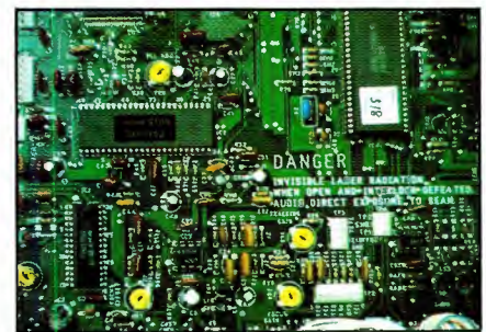
All the servo and laser adjustments and test points are available on one circuit board. The board can be accessed by removing the player's top cover.
