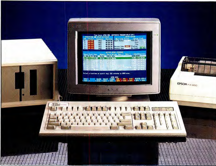
The delay-system screen display should convey clearly the detailed event list, system and VTR real-time activity so that error conditions can be quickly assessed and equipment maintenance procedures planned.
