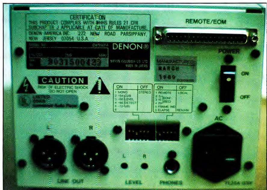
The back panel contains all of the output, power and remote-control connectors. Also available are the DIP switches for selection of operating options.
