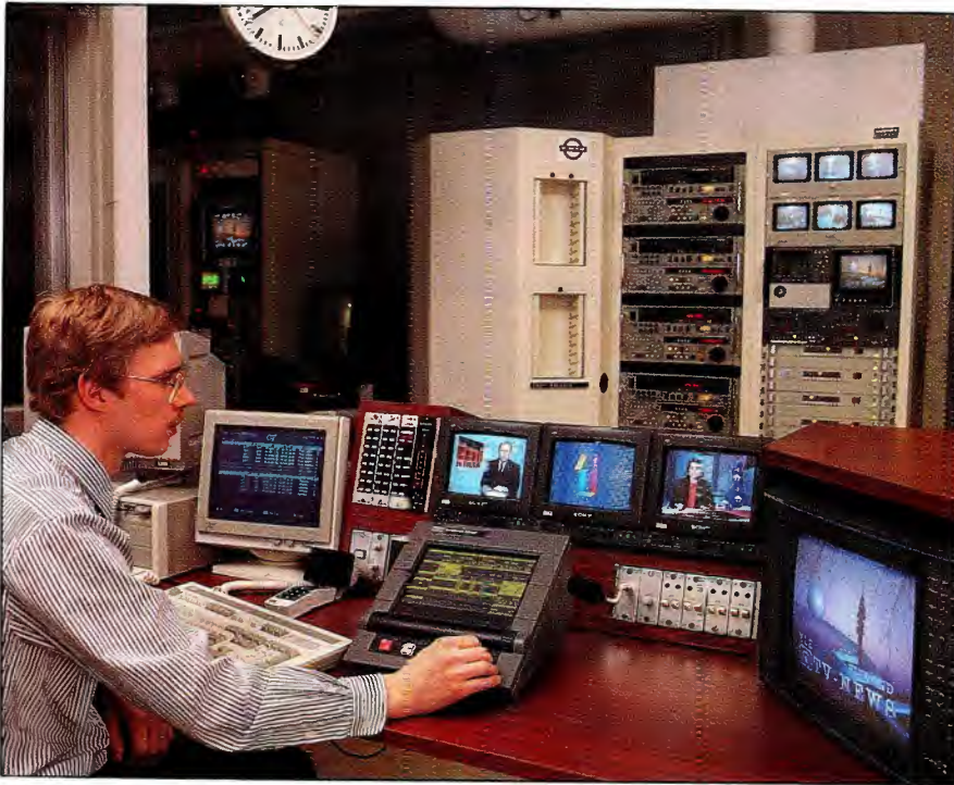
A cart machine remote-control system can simplify news operations by providing instant access to hundreds of tapes and simultaneous control of multiple tape decks.
