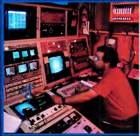
This control room is in a container which was lifted by crane to the deck of Woods Hole's ocean-going research ship. Video engineer Brian Lange uses Sony U-Matic SP equipment to record video sent up by JASON, an unmanned underwater vehicle.
