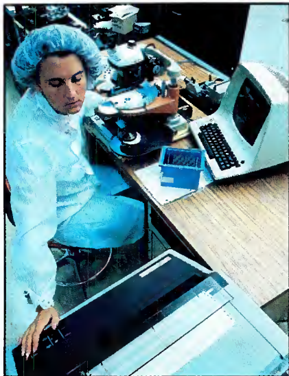
A post-alloy probe of the wafer provides a computerized printout of sample die parameters against specifications. (Courtesy of Precision Monolithics.)
