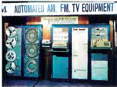
Automation systems have changed dramatically within the past two decades. Shown is the IGM 500 series automation system, which used electromechanical timers for setting up format breaks. An early version of the Instacart can be seen on the left. (Courtesy of IGM.)
