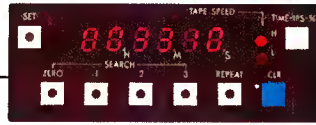
Three cue locations and a zero memory can be accessed via the MX-55NM's built-in locator.
