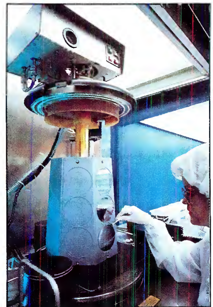
As many as 18 different layers are required to produce the needed circuit pattern on the surface of a typical silicon wafer. Here, an epitaxial reactor grows a single crystal silicon film of the desired dopant concentration upon the silicon substrates. (Courtesy of Precision Monolithics.)
