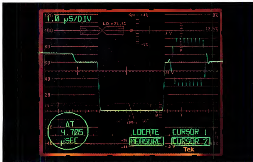
Figure 3. Time cursors, shown here as dots, allow timing intervals to be measured.
