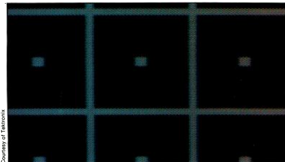
An extreme close-up of the screen shows how groups of dots are illuminated by a convergence pattern.
