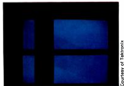
Use of the cross-pulse mode allows the structure of the blanking interval contents to be seen.
