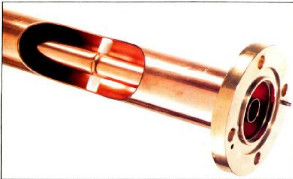
Coaxial transmission line consists of two concentric cylinders aligned on a single axis, insulated from each other.
