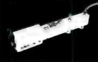
High efficiency space TWTs (including 50 W and 100 W Ku-band for next generation DBS Satellites).
