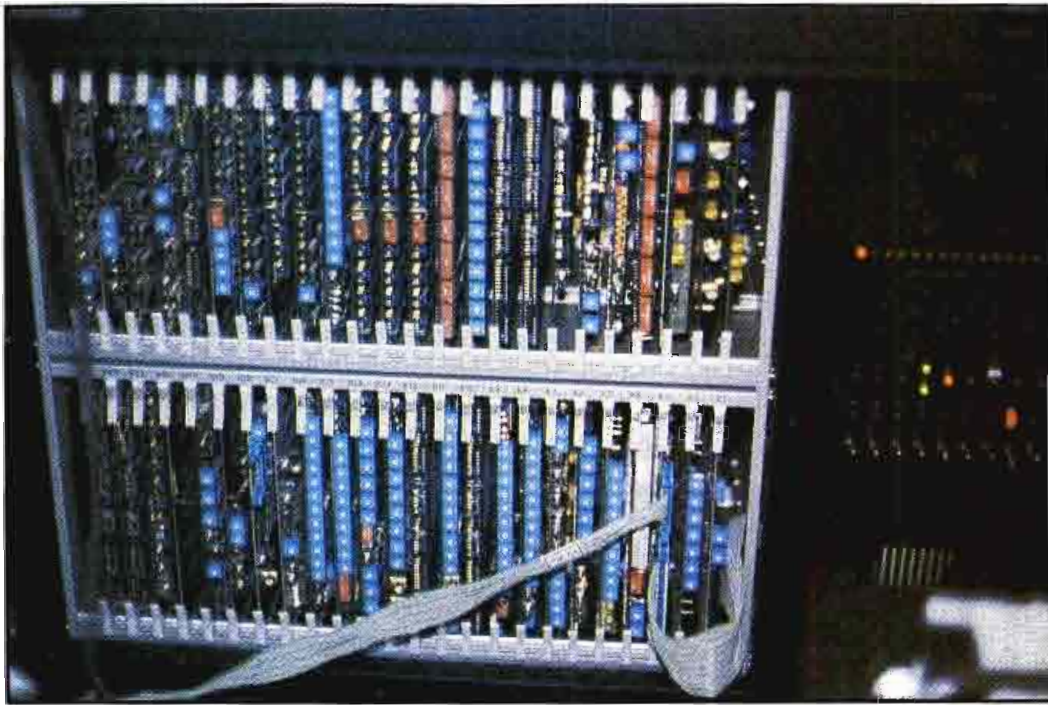
Converting a MUSE signal back to full HDTV bandwidth requires a MUSE decoder. Someday this will be on a single LSI chip.
