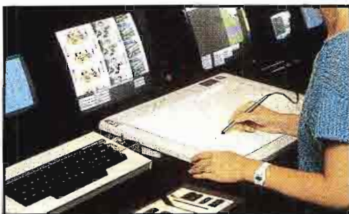
The keyboard, bit-pad and trackball all are available to the artist for control of editing functions on the Quantel Harry, tying the Paintbox and Encore into a digital production system.
