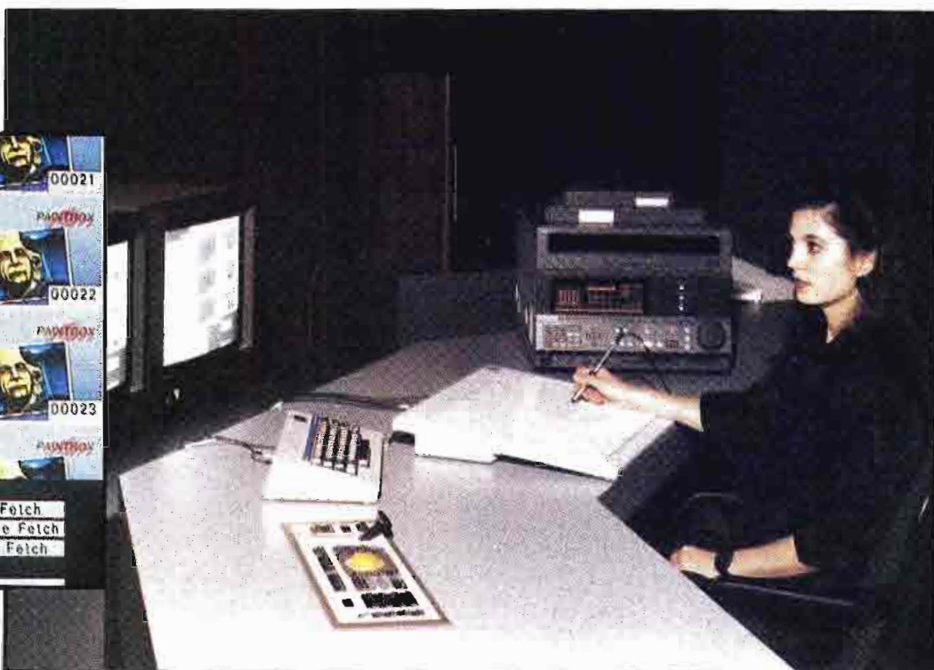
The control screen (see inset) lets the operator choose edit points from several frames from various segments displayed simultaneously. Input is via a light pen.
