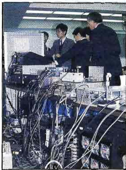
Behind the neatly draped tables in the FCC conference room is a "spaghetti-city" of interconnection among adapters, converters, coders and decoders.
