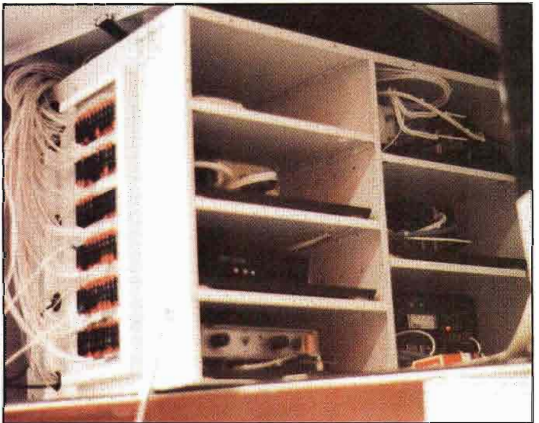
Electronics systems controls from the cockpit are interfaced to the hardware rack in the rear luggage compartment on terminal strips.
