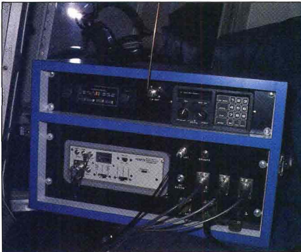
Broadcasting from an aircraft poses special problems for the RPU equipment. The equipment shown here is capable of dual-frequency operation, which provides reliable operation for the station's helicopter traffic reports.
