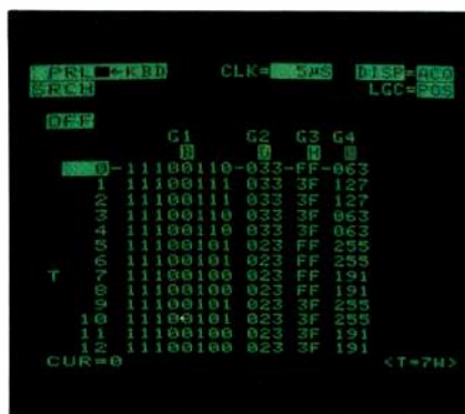
Figure 2. A logic analyzer will display data in a list format when used in the state mode.
