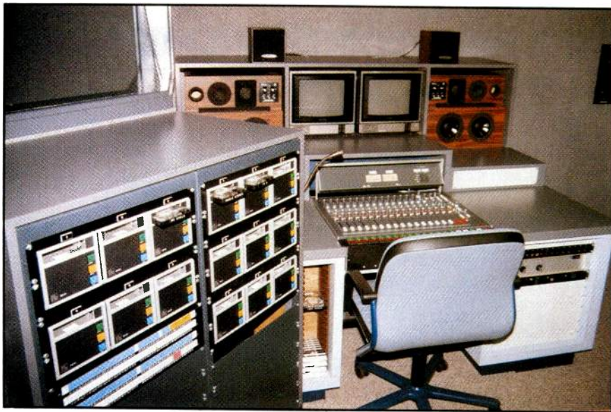
The music room adjacent to the audio mixing room of Studio 4. The music room includes 15 stereo cart machines, a mixer, nearfield monitors and cart storage racks.
