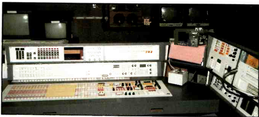
The technical director console under construction in the control room of Studio 4. Video monitors can be seen in the background. A total of 28 black-and-white continuity monitors are used, plus three color monitors (program, preset and preview).
