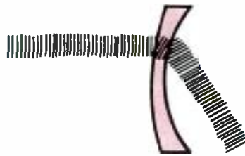
Figure 3. The amount of bending as the light ray enters the lens is determined by the index of refraction of the air and glass. As the ray passes back into air, it is bent again.
