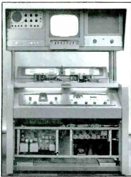
An Ampex VR-1000C VTR with the model 1010 Color Accessory Kit. Note the differences between the VR-1000C and the earliest machine.
