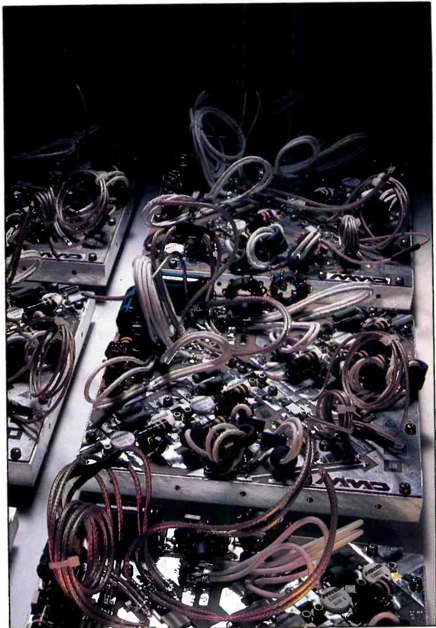
One of the significant developments of the convention was an accelerated move to solid-state technology in broadcast transmitters. Shown above are 600W modules used in several new FM transmitter designs.
