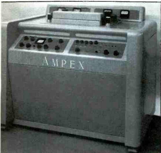
The world's first practical videotape recorder, the Ampex-Mark IV prototype VTR, was unveiled in April 1956 at the National Association of Radio and Television Broadcasters convention.
