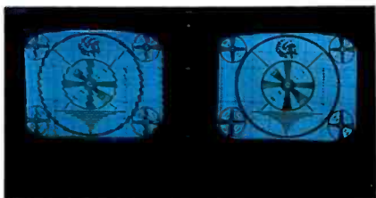
Early VTR engineers constantly had to cope with Venetian blinding (shown at left), caused either by inadequate tip penetration or incorrect head spacing (quadrature error).
