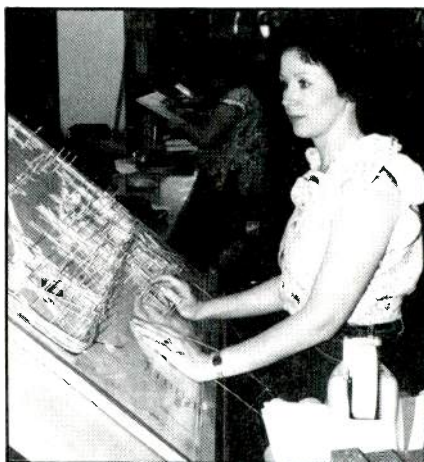
A technician assembles a transmitter wiring harness at a wire harness construction station.
