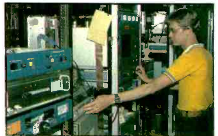
A technician tests the company's new transmitter status video display unit installed in a 3.5kW FM transmitter. The large assembly development lab, where transmitter work is done, is separated from the small signal lab.
