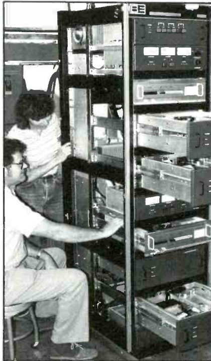
Technicians adjust a 300W dual transmitter before performance testing.
