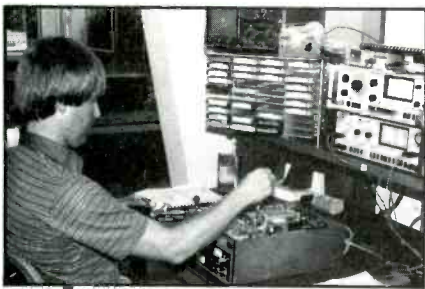
A cartridge tape machine is aligned and tested for proper performance (left). Cart machines are cycled to simulate normal use.
