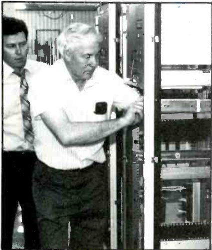
At the medium- and low-power transmitter system assembly area, sub-assemblies and mechanical hardware are combined with wiring harness to form the finished unit.
