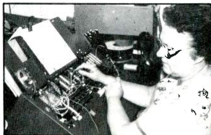
A technician, using wiring harness, combines electrical sub-assemblies and mechanical components to form a finished system.
