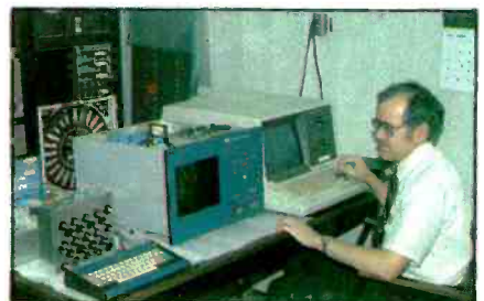
Software development work takes place in a separate area of the engineering lab. Special prototype test fixtures simulate transmitter operating parameters in the development of the CRT status display unit (center).
