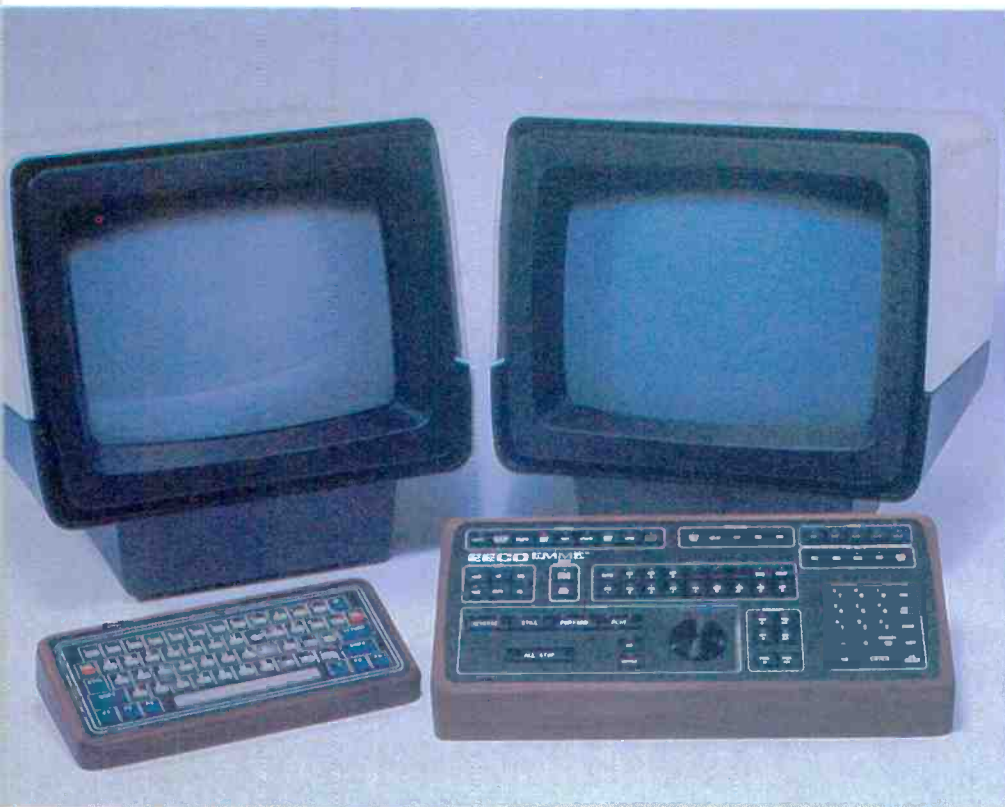
EECO's EMME computer-assisted editing system (independent creative workstation with optional monitors and optional ASCII keyboard shown).
