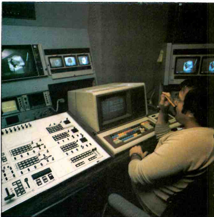
From the ISC editing controller, MTI's Bob Lefcovich handles four VPR-3 machines.
