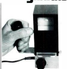
Optical Color Comparator for setting color temperature at all luminance levels, to D<sub>65</sub> or other standards
