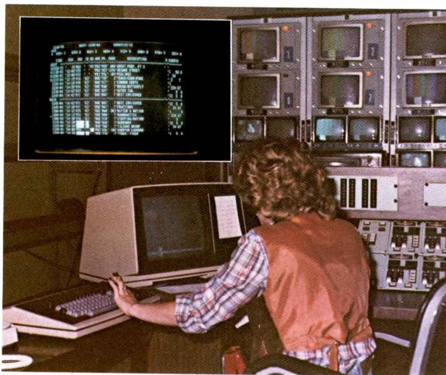
The operator keys commands into the automation system in the master control room. Inset shows a typed CRT display of an event schedule.
