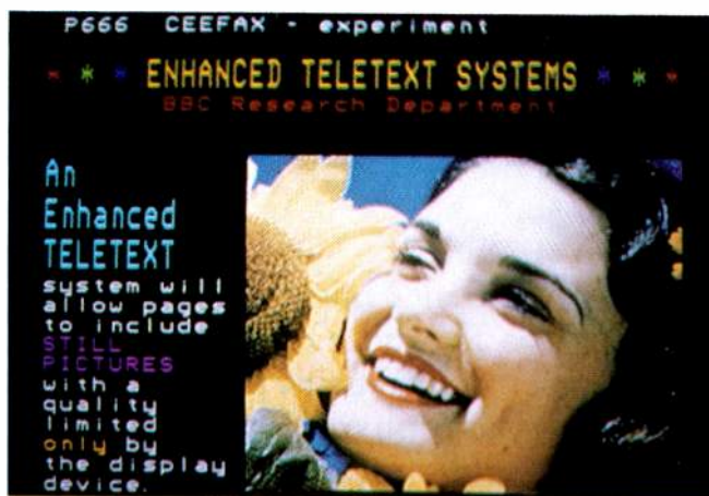
An experimental CEEFAX page incorporating a high quality still picture. (From BBC Research).
