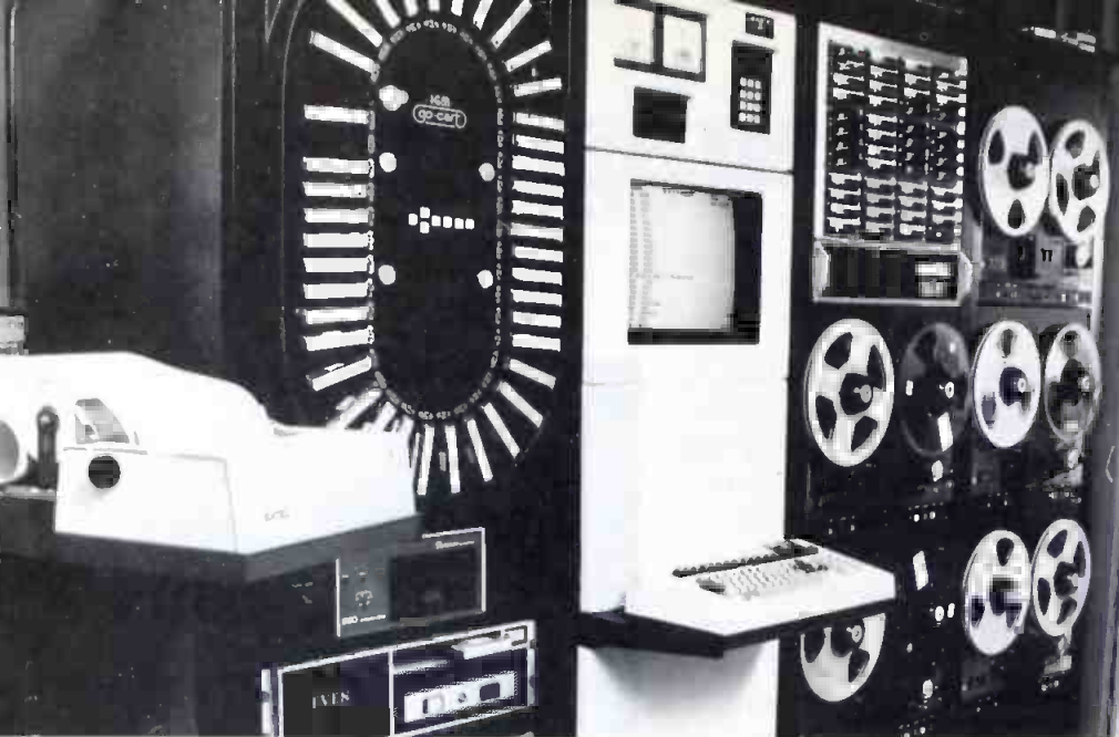
Figure 1. The BASIC A audio control system utilizes three separate microprocessors to handle commands, control functions and print out the records. The article here describes engineering decisions behind the design and development of this system from concept to finished product.
