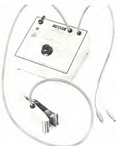
Fig. 4 A logic monitor clips on IC pins to show operation of each pin simultaneously. This attached logic monitor can be used on all logic families. (Photo courtesy CSC)
