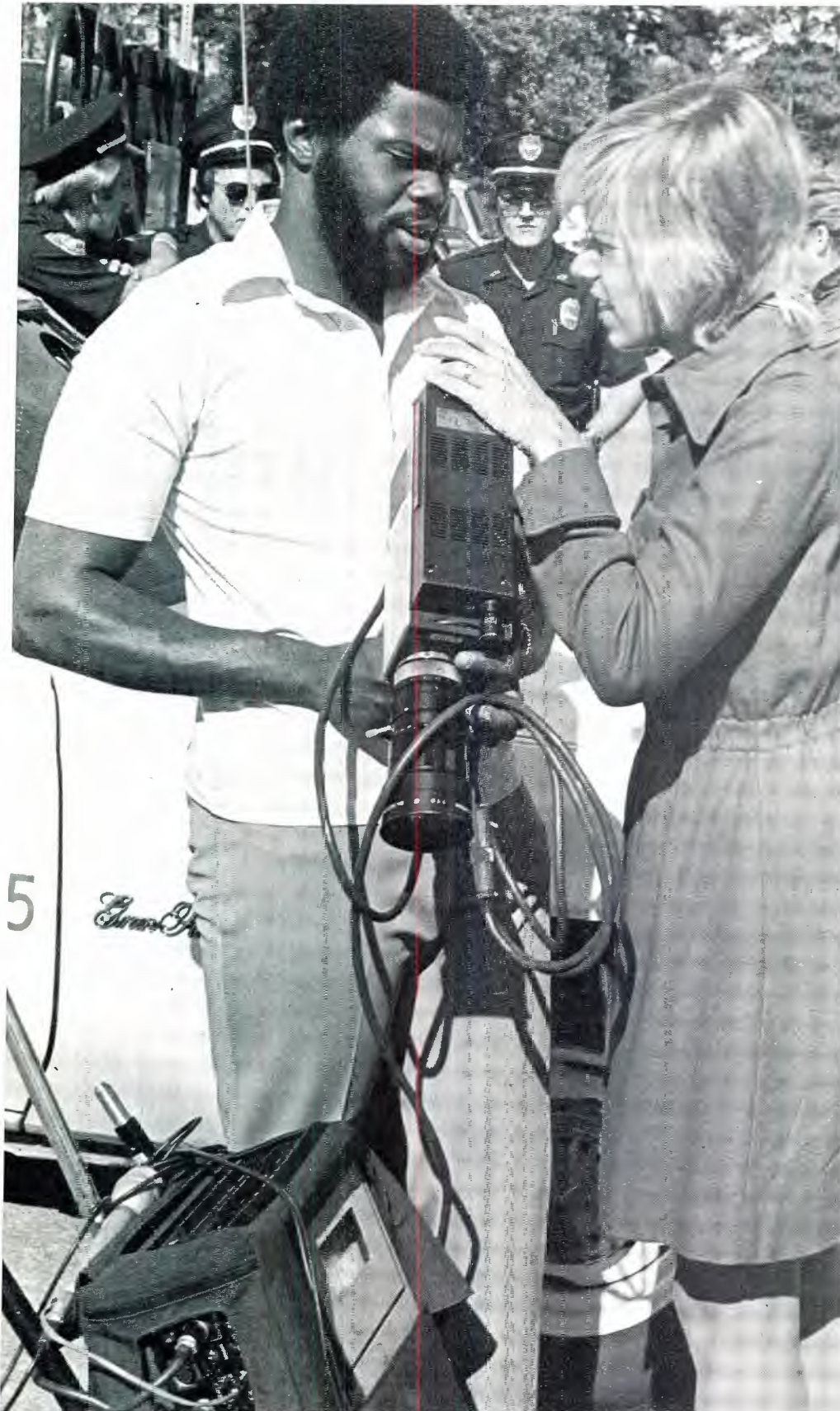
With ENG, stories can be immediately checked in the field by playing the tape back through the viewfinder. Cameraman Tony Cunningham and news reporter Jan Gauss check the playback of a civil disturbance story they've just covered.
