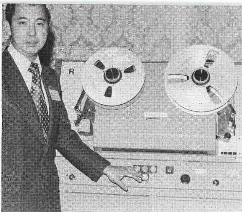
Recortec president Dr. Lester Lee is shown here with a VR1100 fitted with constant tension transport modifications and a digital readout timer manufactured by his company. Dr. Lee delivered a paper on updating quad VTR's.
