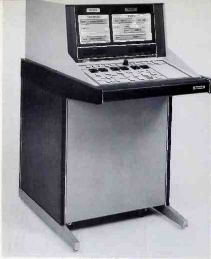
Fig. 3 The DOZ have installed two Ampex RA-4000 automated programming editors that use the newly developed address code editing technique. Each frame is assigned a specific number that can be selected by visual readout or by digital pre-selection.
