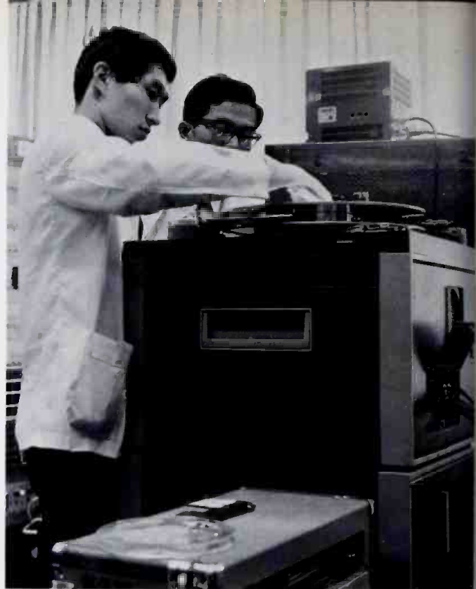
Fig. 4 The slow motion disc recorder shown here was used by the NHK at the Mexico City Games. This was the first use of color slow and stop motion disc recording at an Olympiad.
