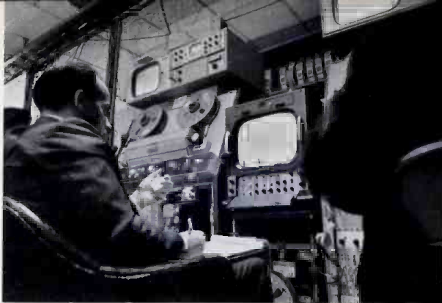
Fig. 2 A typical Olympic setup for electronic editing of daily events into completed evening program for transmission. Conrac monitors are used in this shot for picture quality control.
