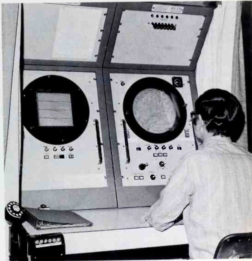
Fig. 4 Travelers Weather Service Terminal. Display at left is the Range Height Indicator (RHI) and at right is the Plan Position Indicator (PPI).
