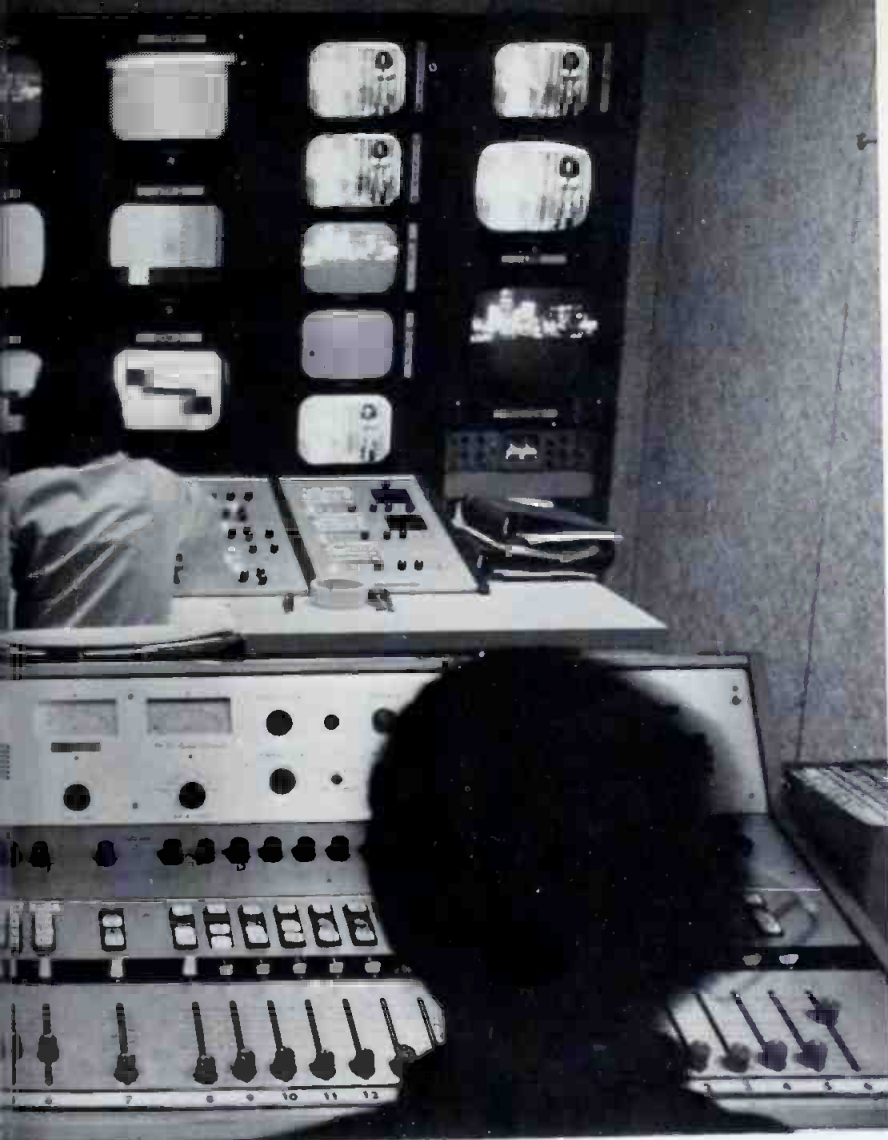
Fig. 1 Four separate control areas, two for production and two for air broadcast, are provided and allow the three studios to be linked together in any combination through a separate master control.
