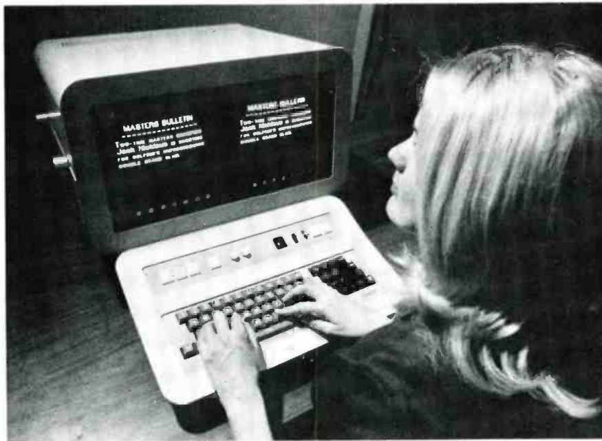
Fig. 2 Vidifont system is operated by a typist who punches out programming information as needed.
