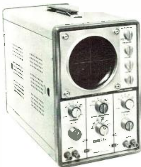
The EICO 465 is an easy-to-build kit scope. The power supply has gone solid state, while the amplifiers are still tube-type.
