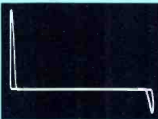
Fig. 3 Waveforms typical of most normal germanium transistors. (A) PNP polarity transistor with base connected to H and emitter (or collector) to G. A diode with the cathode connected to H and the anode to G will produce the same waveform. (B) The same PNP transistor with the base connected to G and the emitter (or collector) to H. A diode with cathode to G and anode to H produces the same waveform. (C) A PNP transistor with the emitter connected to H and the collector to G. Rectification is inefficient, and scope gain must be increased to obtain a large waveform.
