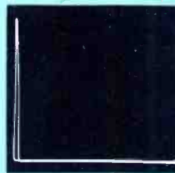
Fig. 3 Waveforms typical of most normal germanium transistors. (A) PNP polarity transistor with base connected to H and emitter (or collector) to G. A diode with the cathode connected to H and the anode to G will produce the same waveform. (B) The same PNP transistor with the base connected to G and the emitter (or collector) to H. A diode with cathode to G and anode to H produces the same waveform. (C) A PNP transistor with the emitter connected to H and the collector to G. Rectification is inefficient, and scope gain must be increased to obtain a large waveform.
