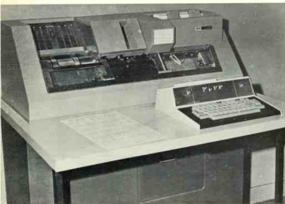
Fig. 2 IBM keypunch machine for punching codes to represent alphanumeric characters by combination of holes.
