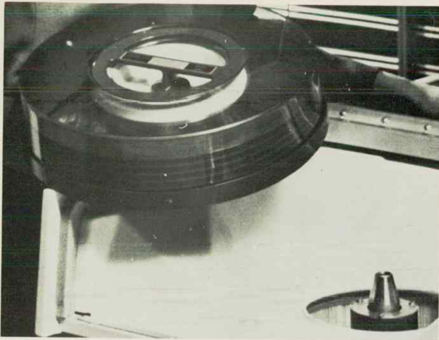
Fig. 1a Typical computer I/O devices include the magnetic disk pack.
