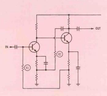
Fig. 5. Second transistor acts as an emitter-circuit "electronic choke."
