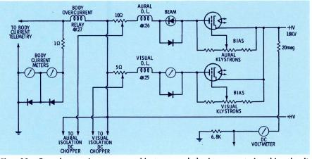
Fig. 12. One-ohm resistor senses klystron and body current in this circuit.
