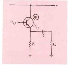
Fig. 4. Part of output signal current is diverted through emitter resistor.
