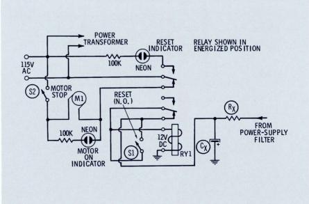
Fig. 1. Circuit of generator with a fast-acting failsafe provision.
