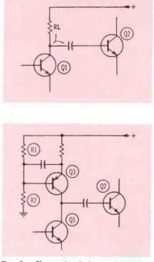
Fig. 8. Electronic choke replaces R<sub>L</sub>. BROADCAST ENGINEERING
