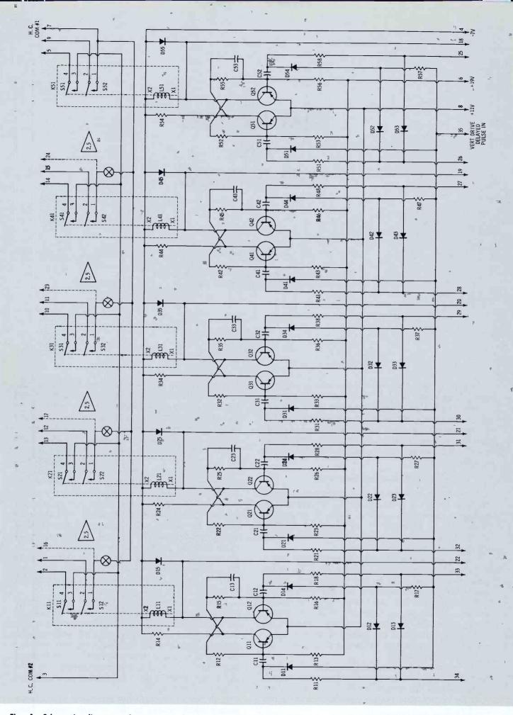
Fig. 1. Schematic diagram of one vertical-interval control card relates five identical flip-flop and relay circuits. 12 BROADCAST ENGINEERING
