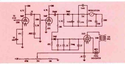
Fig. 15. Additions to studio monitor are used to monitor audio modulation.
