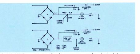
Fig. 11. Sensing circuits employed to measure aural and visual frequencies.
