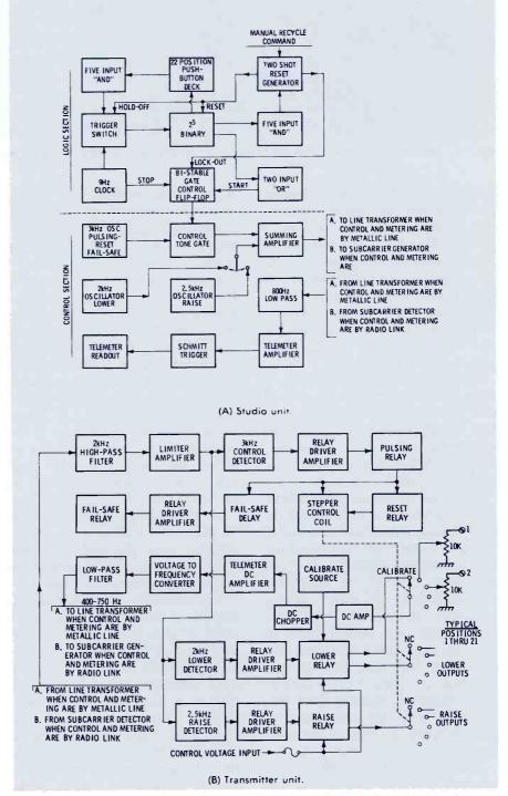
Fig. 2. Block diagram of the Moseley PBR-21 remote-control unit with changes.
