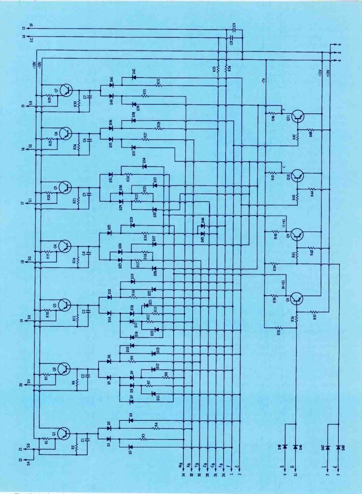
Fig. 2. Logic-card circuit indicates diode gates, emitter followers Q1 through Q7, and inverters Q8 through Q11.
