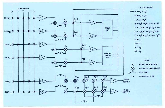
Fig. 4. Typical switching matrix for system including fader and special-effects units with useful logic equations.
