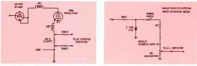
Fig. 13. Driver-modulator sensing circuit uses chopper.
