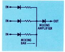
Fig. 10. Typical audio mixing method.
