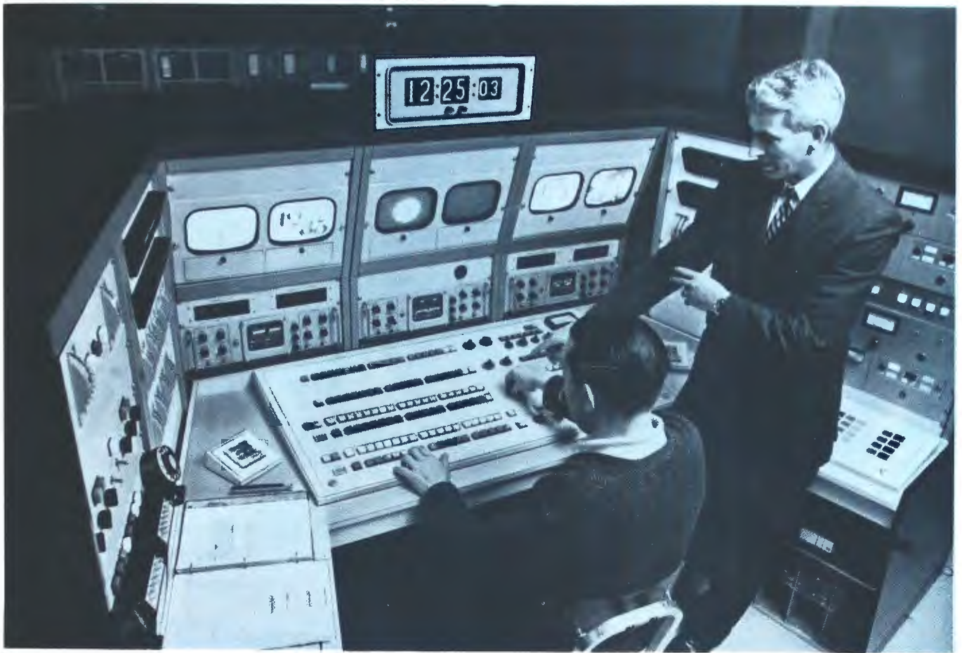
Typical of the customized concept in Visual solid-state Video Switchers is this system installed at WHYY-TV, Philadelphia. Used for switching Channels 12 and 35 WHYY's Master Control Switcher incorporates preset 16-event store, audio-follow-video and audio breakaway facilities, independent switcher busses to five VTRs, program and preview feeds, full machine control, and audio-video monitoring and preview facilities.
