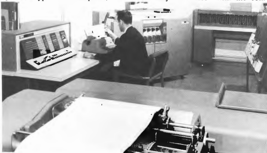
Operator, console are at left, card reader in rear, printer in foreground.
