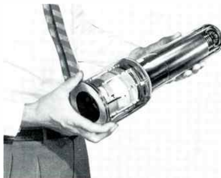
This is the big 4-1/2 inch I.O. tube for sharper pictures.
