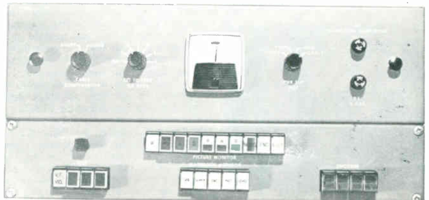
Power supply for the PE-250 is at the camera control-unit position.
