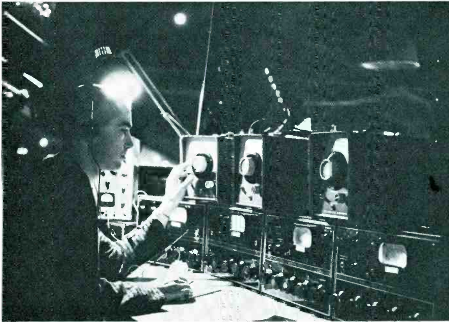
Fig. 2. Setup of several receivers used for political or indoor sports coverage.
