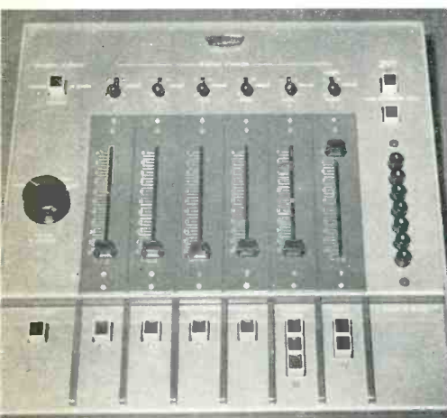
Fig. 2. Completed switcher console panel.
