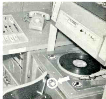
Fig. 3. Rear view of announcer's position shows turntable switches and cue speaker.
