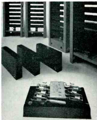
Fig. 1. A typical module of the high-v silicon rectifier assemblies (background).
