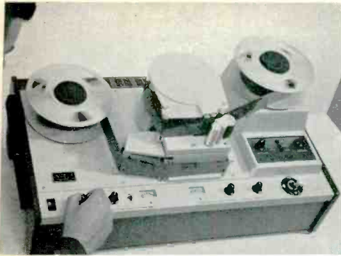
Fig. 6. This helical model employs 2" tape and has a "joy-stick" tape motion control.
