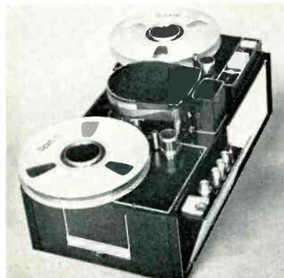
Fig. 5. A helical recorder which uses 1" tape and plug-in circuit board modules.
