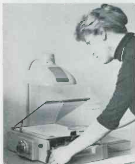
The frames from the traffic board are inserted into a Kodak Verifax Signet Copier. Reproductions of the information on the frames is made by exposing the frames to a light-sensitive matrix paper.
