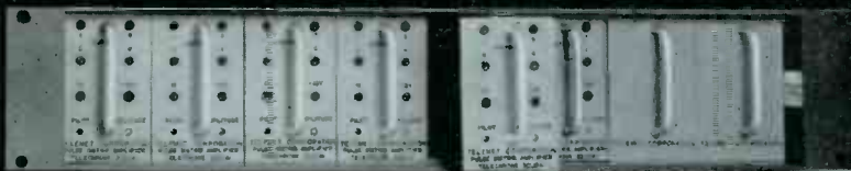
MODEL 3202 PULSE DISTRIBUTION AMPLIFIER. Output level adjustable between 3.5 and 4.5 volts; output pulse within EIA specs and constant over an input voltage range 1.5 and 5 volts; failure alarm indicates loss of output pulse
