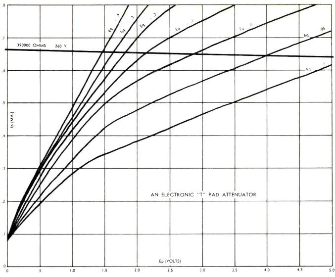
Figure 2 Plate characteristics of one section of a 12AU7 tube.
