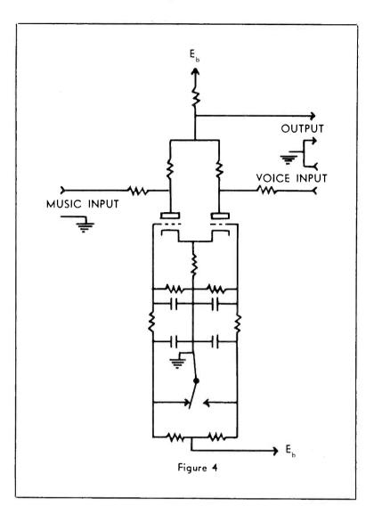
Relay controlled duplexfader os used in automatic program installation.
