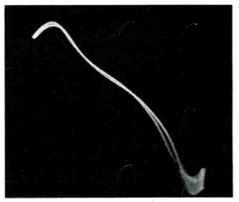
Fig. 6—With a typical misaligned discriminator such as this, there is no way of tuning in a station so that the subcarrier sidebands will balance each other. As a result, unwanted demodulation of the subcarrier will be heard along with the regular main channel program,
