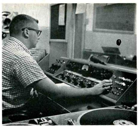
The push button control console built at KHJ which enables the engineers at KHJ to have instant cueing and split second control of all program material.
