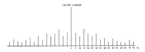
Figure 1—With 5000 cps modulation on the FM transmitter, sidebands are generated at intervals of 5 Kc. above and below the carrier. Audio tones of other frequencies will produce sidebands spaced in accordance with the frequency of the tone. The amplitude of the applied tone determines the extent of the deviation and the amplitudes of the individual side carriers.
