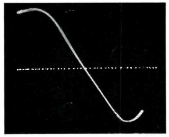
Fig. 3—Correctly adusted discriminator or ratio detector produces this type of "S" curve. With a variable marker oscillator the length of the linear slope can be measured. It should be at least 200 Kc. for low distortion as well as for minimum demodulation of the subcarrier audio.
