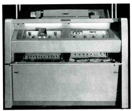
Front panels of VTR console dropped down, revealing easy accessibility of controls used by the operator in routine maintenance adustments.
