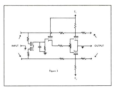
Electronic balanced "H" pad used in Broadcast Remote equipment.
