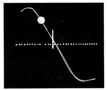
Fig. 5—The large white dot is placed to show the position of the main carrier when the receiver is tuned to one side. Only one of the 65 Kc. sidebands appears on the linear slope. The other one is lost. In this case, the sideband which appears on the slope will be detected as it deviates with modulation. The shorter the linear portion of the slope is, the more exaggerated will be the condition.
