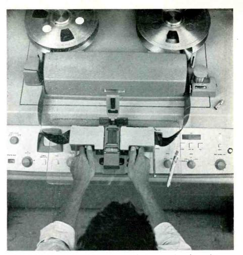
Operator splices TV tape with videotape splicer mounted on front of Ampex videotape television recorder, directly above console's control panel.
