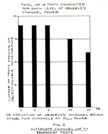
to each of the three TV receiver antenna terminals for 70 watts peak visual output from each of the transmitters. Approximately equal signal strengths were available from each of the transmitters at the terminals of all three antennas,
