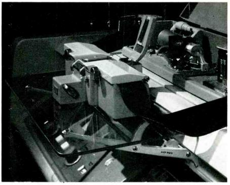
Closeup view of videotape splicer mounted on front of VTR console directly above control panel.
