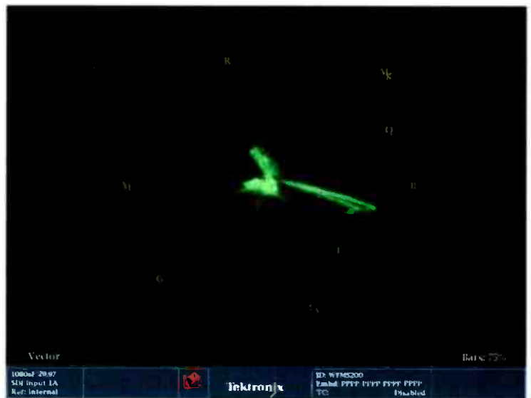
Figure 3. A vectorscope is an XY plot of color (hue) as an angular component of a polar display, much like some familiar color wheels used in color graphics.
