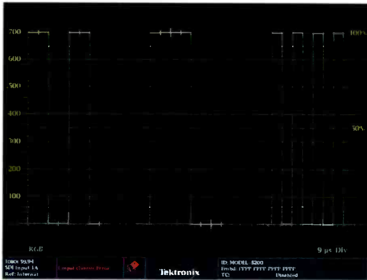
Figure 2. The most common type of parade waveform displays, the RGB Parade, shows the red, green and blue channels of color.
