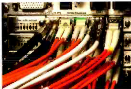
Figure 1. SFP technology allows for mixed-mode operation of both coax and optical in large 3Gb/s routing switchers.
