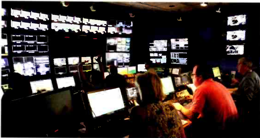
Nearly 50 new LCD monitors, including a mix of 32in, 46in, 60in and 85in displays, help the CBS Sports Network staff produce shows and more than 350 live games each year.
