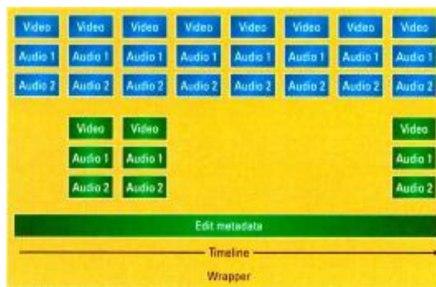
Figure 2. An AAF file could contain a base layer, a compositing layer and some editing metadata,
