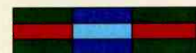
Figure F: Interpolated blue value where there is only a green sample
