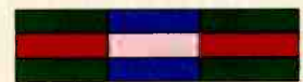
Figure D: Interpolated red value where there is only a green sample
