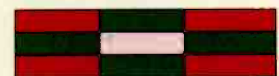
Figure E: Interpolated red value where there is only a blue sample
