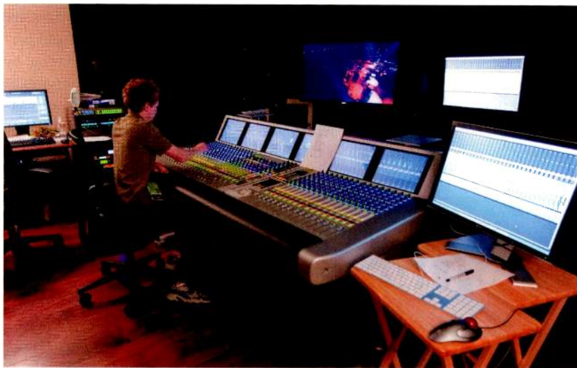
The S5-BP's Expand Tracks function lets "ACL" video editors, who cut the show on Media Composer, quickly conform Pro Tools tracks from the recorded concerts to match the picture edits.
