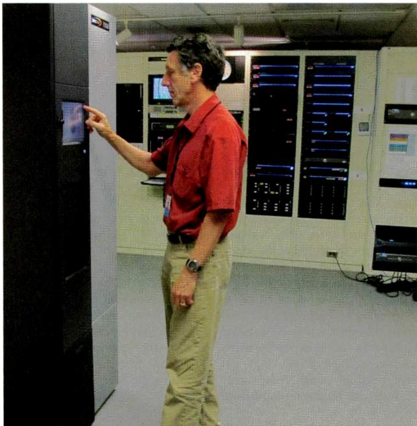
Bruce Jacobs, CTO of Twin Cities Public TV, uses Spectra's BlueScale 11 operating system to check the status of the Spectra T950 tape library.
