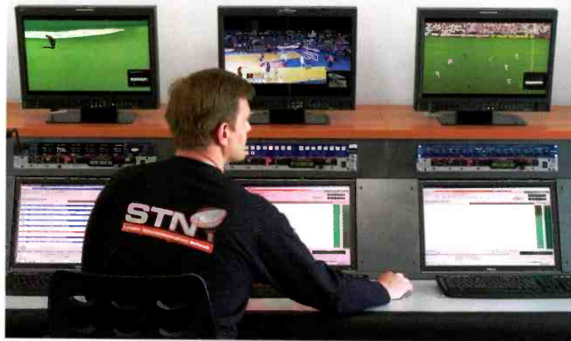
Satellite Telecommunication Networks (STN) in Slovenia monitors loudness with Jünger Audio's Level Magic. The system features an adaptive level control algorithm capable of adjusting the right audio level from any source at any time.
