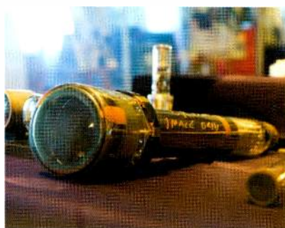
Photo 2. Early engineering model of the image orthicon pick-up tube
