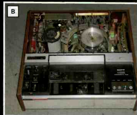
Photo A: Ampex demonstrates the VR-2000 server, circa late 1950s. Photo courtesy Ampex/Wayne E. Carlson. Photo B: Sony's VP-1000, circa early 1970s, was a first-generation U-matic top-loading, play only deck with basic functionality. Photo courtesy LabGuy's World. Photo C: In 1935, German company Allgemeine Elektrizitätsgesellschaft (AEG) in Berlin developed the AEG Magnetophon. Photo courtesy EMTEC Group.
