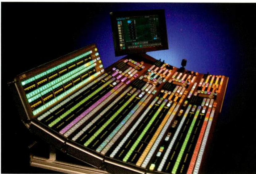
Grass Valley's Kayenne switchers offer broadcasters 1.5 to 4.5 M/E, with unique functionality, such as six keyers per M/E.
