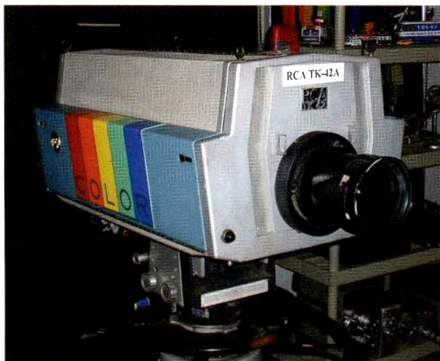
The first 60 units of RCA's TK-42 camera were delivered in 1965. The camera featured a 4 1/2in image orthicon tube and three 1in Videocon tubes. Photo courtesy Bobby Ellerbee.
