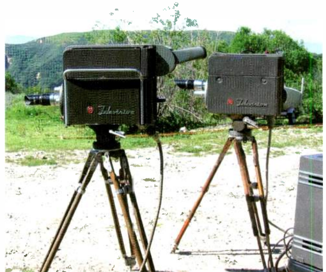
RCA's TK-30 and TK-31 were introduced in 1946 and used during the 1950s. Photo courtesy Chuck Pharis.
