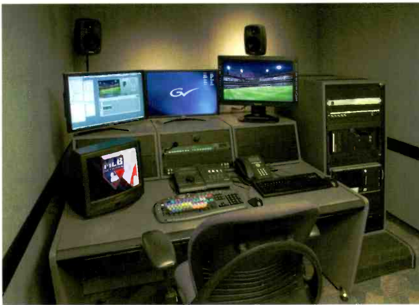
The facility includes 15 HD edit suites equipped with Thomson Grass Valley Aurora news editing software responsible for turning around content fast. The HD suites are seamlessly connected to a Grass Valley storage area network.
