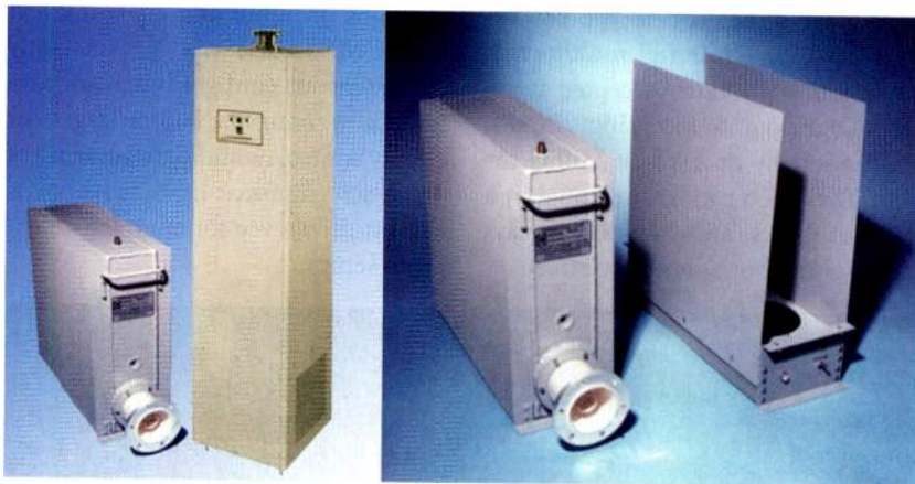
Figure 1. This illustration shows the oil load vs. forced air. The relative sizes of an oil load with a 3-1/8in EIA flange connector are shown on the left, and a forced air load is shown on the right. The right panel contains the same oil load with an optional cooling fan and shroud to extend the power rating above 5kW.
