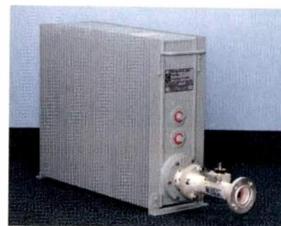
Shown here is a completed high-power attenuator assembly using a lower power 1-5/8in rigid line with EIA flanged connectors and coupling section. Not shown are the 1-5/8in to N, LC, HN, 7/16 or between series connector and adapter that can be added to the line section input. The attenuated output is available from the top of the element in the center of the line section. An optional BNC attenuator can be used to achieve higher attenuation values.
