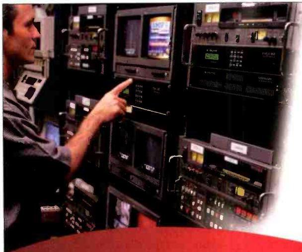
Miranda's Kaleido-X multiroom, multi-image processor was recently installed in Télé-Québec's production control area.
