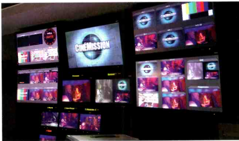
Miranda's Kaleido-X multiroom, multi-image processor was recently installed in Télé-Québec's production control area.
