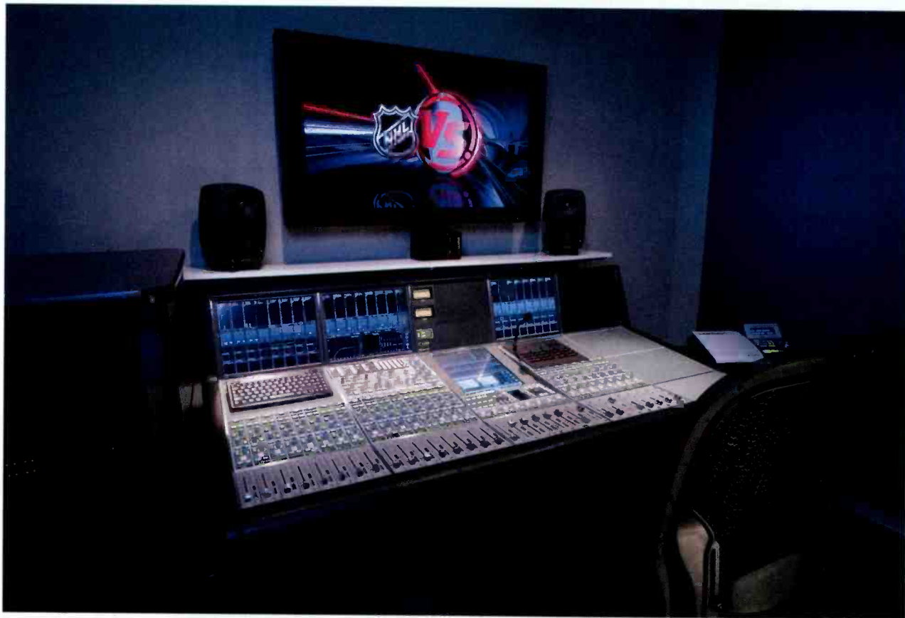
An SSL C100 HD broadcast console is the central piece in Versus' HD audio production.
