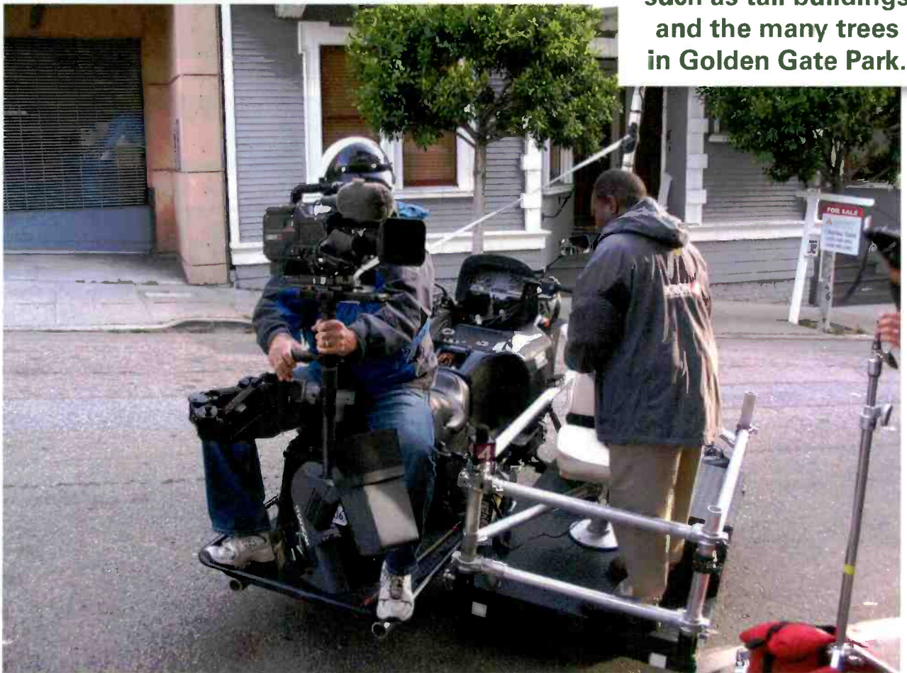
To cover the "ING Bay to Breakers" race, a motorcycle was custom-equipped with a portable high-power transmitter, RFX-PHT, and two antennas mounted onto a pole. The motorcycle carried cameraman Jack Uhalde and reporter Vernon Glenn along the race trail.
