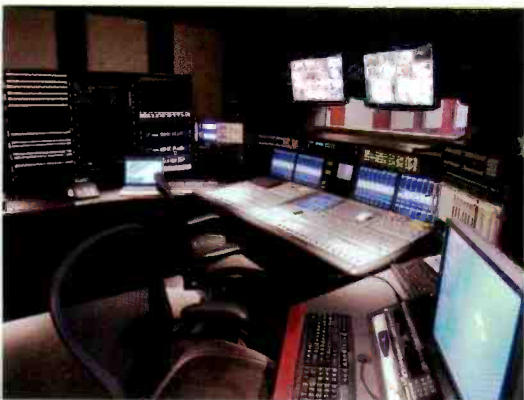
The WETA digital audio control room employs an SSL C100 5.1 surround-sound console.
