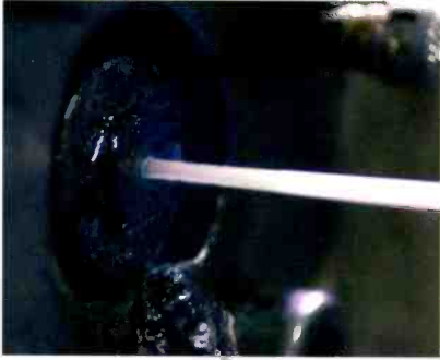
Shown here is a gas-injected dielectric expanding as it is extruded.
