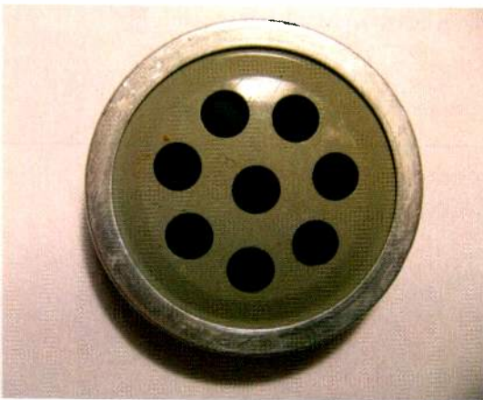
In carbon microphones, carbon granules are placed between two metal plates. Sound waves cause the carbon to compact, which changes the resistance. This converts sound waves to voltage fluctuations.
