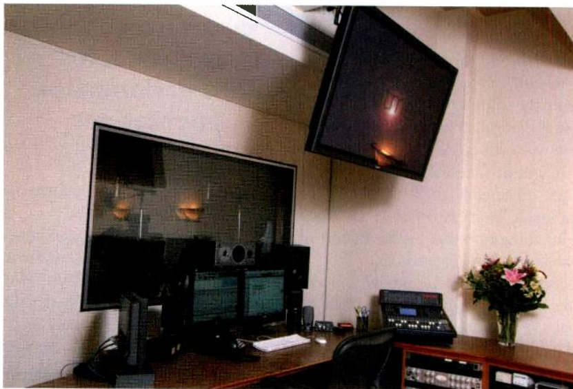
The Yamaha DM1000 console offers Nutmeg Audio Post calibrated monitoring level control. The unit also saves space with its included HUI emulation.
