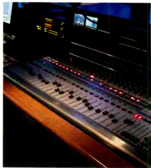
A Wheatstone D7 digital audio mixer is the digital audio control center for the system. It uses a common electronics frame located in the equipment room and has a control panel located in each of the two identical production control rooms assigned to separate studios.
