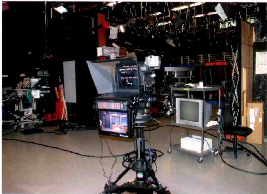
Autoscript's TFT17HB 17in High Bright teleprompter is integrated with a TallyPlus camera numbering system, which has a large LED indicator, and a ClockPlus SMPTE time-code clock.
